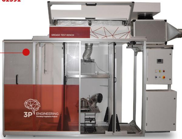
according to specific regulations (variant of the measurement of ORF-Odour Reduction Factor, IEC/EN 61591 referring to the EN 13141-3 European standard about residential ventilation), to study possible interferences on the hood operation.
