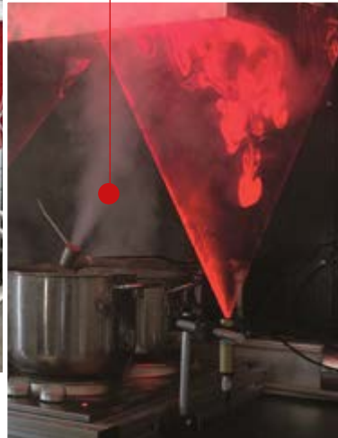
Capture efficiency tests in 3P Multi function Testing Chamber
